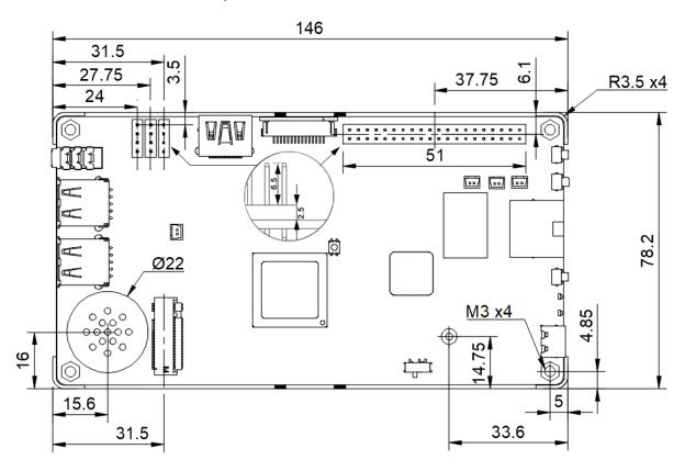
Your expansion board does not need to match the exact dimensions of the Vivid Unit; however, to secure installation, it should utilize at least one of the four mounting holes provided on the Vivid Unit.
