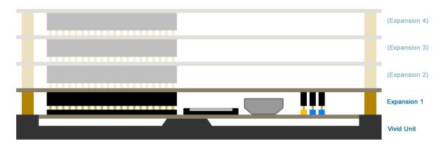
However, a potential drawback is that the final device may become quite thick due to the height of the stacking headers. Additionally, the stacking headers occupy a significant area near the edge, which may complicate or even prevent certain applications.
