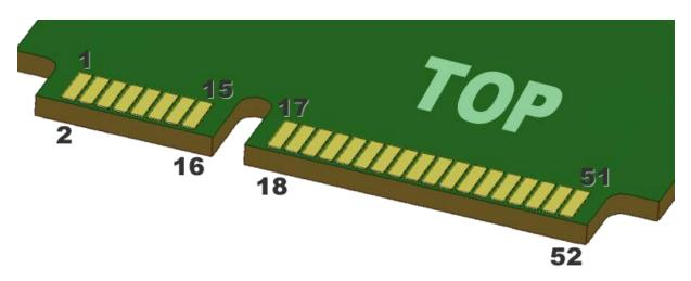
The expansion board connects through 52 edge contacts, as shown in the pinout diagram below:
